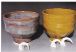
Some glazes that contain iron can change color if fired twice. The extended heat work changes the color and sometimes the surface too.
