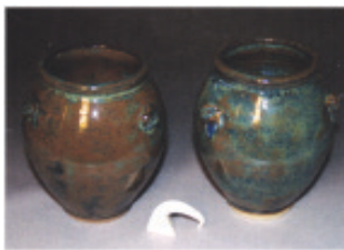
The same glaze can look different when applied on different clay bodies. Iron in the darker clay (left) reacted with the glaze and changed its color.
