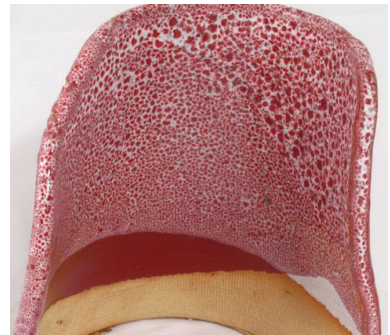
Another test on the right with Marshmallow (CG153) dipped over Brick Red (CG142). Spots become noticeably larger and less regular after each new coat of glaze.
