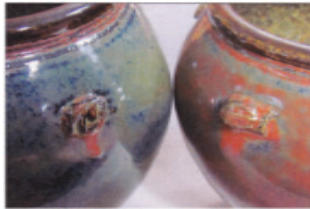
Same glaze: the left bowl had a thinner application and 14 hours firing. The right bowl had a thicker application and faster firing (9 hours).
